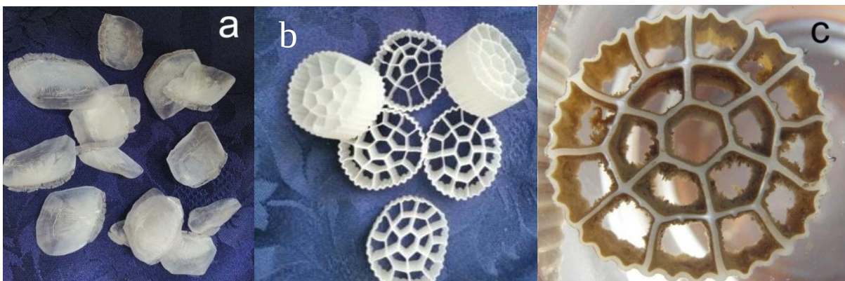
Figure 3. Types of carriers used in the study : (a) scales of Umbrina roncadore used as a natural support, (b) industrial Kaldnes K3 carriers before colonisation, and (c) after colonization by the biofilm.
