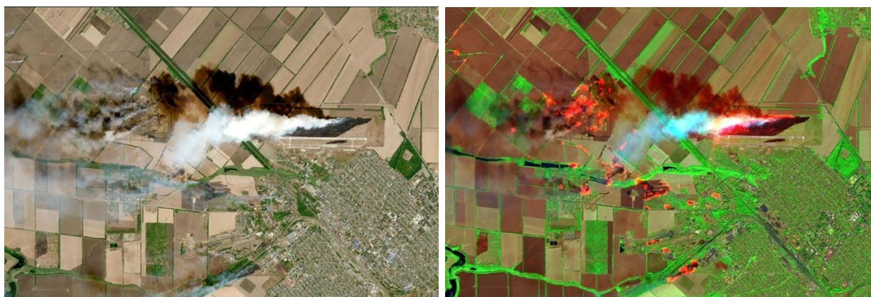
Figure 15: Sentinel 2A satellite images of ammunition depot and military airfield near Tikhoretsk taken on 21 September 2024: above in natural colour; below, combination of B12, B8 and B3.
