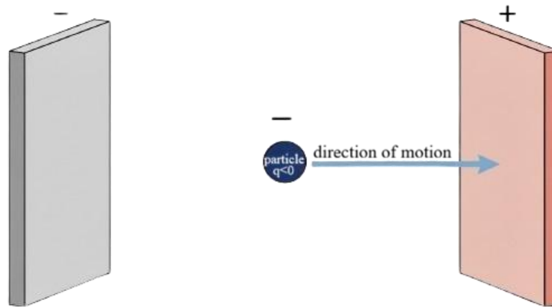
Figure 4. Migration of a charged particle in an electric field
