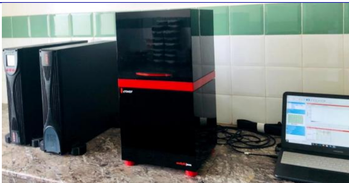
Figure 2. Real-time RT-PCR workstation used for quantitative detection of SARS-CoV-2 RNA and monitoring of cycle threshold (Ct) values for the RdRp and S gene targets under different storage conditions.
